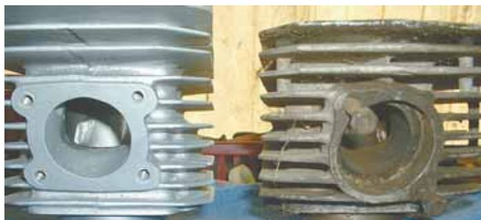
Bead blaster uses no. 80 glass beads to remove rust, oxidation and corrosion without damaging metal parts.
