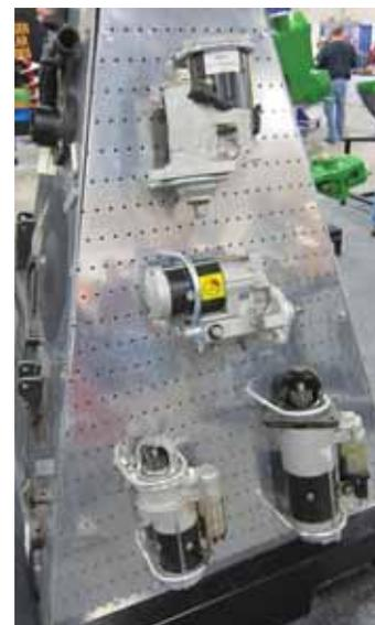
Abilene Machine's 24-volt to 12-volt conversion kit for Deere tractors includes a gear reduction starter.
