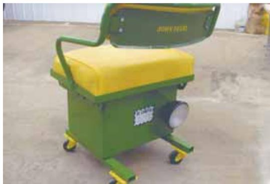
Rolling shop chair was made by mounting the seat and battery box off an old Deere tractor on a set of swivel caster wheels.
