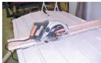
blade cuts plastic, steel, aluminum and wood with one blade. It's great for working with reclaimed wood. If you hit a nail, it cuts right through it.
