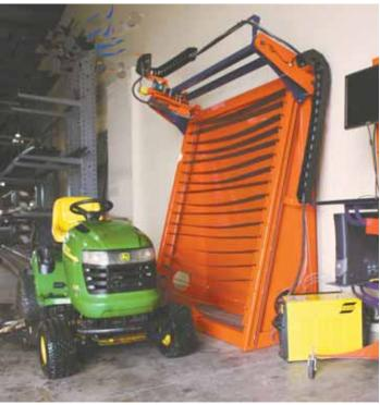
BurnTables vertical CNC table takes up only a 26-in. strip of floor space, yet can handle up to 60 by 60-in. sheets of material.
