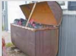
"I made a dumpster out of an old fuel tank. It stands on wood blocks and I hinged the top 1/4 of the tank, putting a handle to lift it. Metal rails tack-welded to top edge reinforce the tank and cover the sharp edges."
