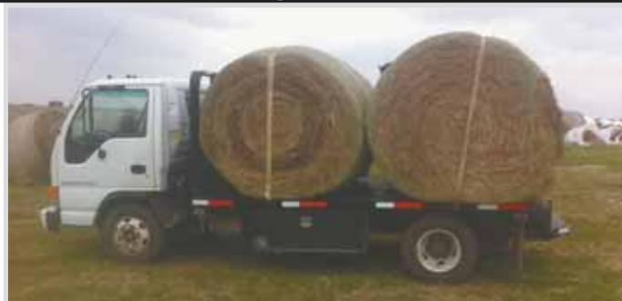
Stevens removed the cargo box from an Isuzu truck and fitted the frame with a flatbed off a 1-ton Chevy.
