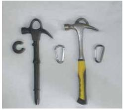
One looped hammer has a crows foot prybar at the bottom; the other is a steel claw hammer with comfort grip.
