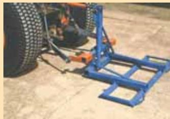
Home-built, 3-pt. mounted service lift lets Jerome Webb work under his riding mower without removing the deck. A pair of square lift frames support mower's front wheels.
