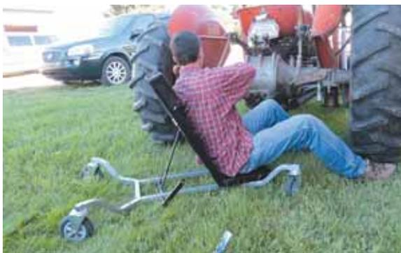
All-terrain creeper has large pneumatic wheels and a reclining seat that can be set at different angles.
