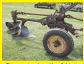
This was originally an IH no. 8, 1-bottom moldboard plow. The 15-in. dia. auger, along with a 3-speed transmission and a pair of pto shafts, was added by Service Equipment of Dallas, Texas. The transmission was the same one found on the Farmall F12 tractor. At the show I pulled the plow around with a Farmall M.
