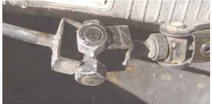
Fred Davison turns nuts and bolts into hinges, universal joints (above), wire tensioners, corner post braces and more.
