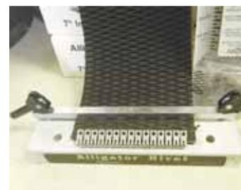
Mark Burrell says his Flexco Alligator Rivet Tool can be used to fix a baler belt in minutes, without the need for a vice or tool bench.
