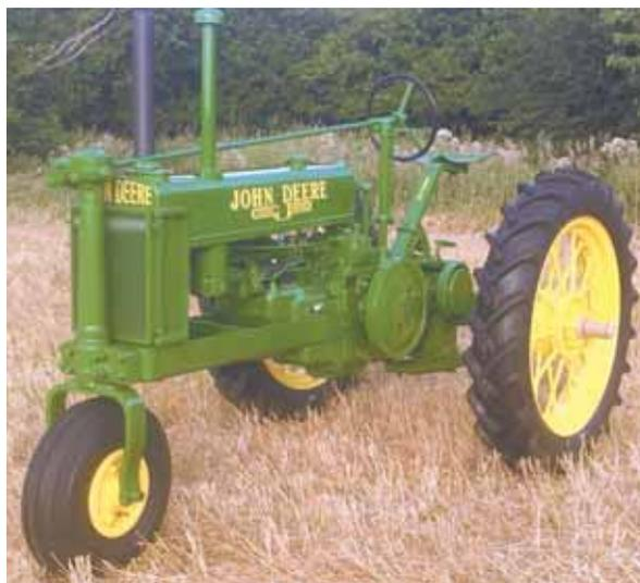
The exhaust stack on this tractor was coated with black ceramic. Ceramic coatings can handle high heat without discoloring, says K&A Coatings.
