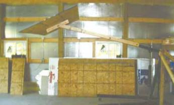
He bolted an 8-ft. long 2 by 4 along each side of the boom, then angled a 2 by 4 between the ends of the boards and screwed on a 12-in. sq. piece of plywood.
