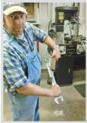
Larry Klavemann, Wilton, Iowa: "I needed a cheater bar to put more leverage on my big wrenches. So I cut and welded two small pieces of angle onto a length of square tubing so I can easily slip a large wrench into it. Easy to use and I get a lot more leverage."
