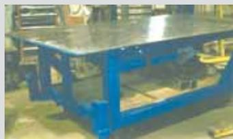
**John P. Vandenbosch, Seymour, Wis.:** "I built a very heavy-duty workbench using the frame of an industrial air conditioner that's made with 4-in. sq. tubing with 1/4-in. sidewall. The top is a piece of 3/4-in. thick 60 by 120-in. plate steel. It's fitted with 2 castor wheels and two standard wheels and has two stabilizer legs, a tongue for moving, and 4 steel drawers made from scrap sheet metal. It weighs a little over a ton and is practically indestructible."
