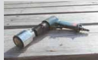
building a new hay rack and had to drive in a bunch of 6-in. long 60D nails. Driving all those nails with a maul got tiring real quick. So I came up with the idea of using an air chisel that came with a planishing hammer. The shaft happened to fit through a 3/4-in. drive by 1 1/2-in. socket. All I had to do was hold the socket on the nail and drive it in. Worked great."
