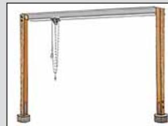
**Lawrence Schaub, Belle Fourche, S. Dak.:** "I used two 5 by 6-in. treated poles 11 ft. high in my shop to support a 12-in. steel I-beam running from one side to the other. Then I fitted an overhead trolley to lift heavy equipment, such as rear wheels off a tractor. The chain hoist I use will lift 2,000 lbs. Very simple and handy."
