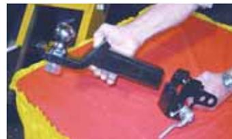
One end of bracket slides onto receiver hitch tube, and the other pins onto the receiver hitch base on the vehicle.
