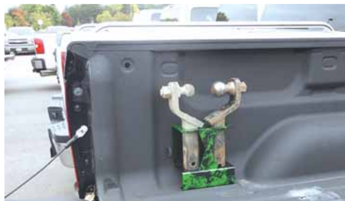
The Pro Hitch Caddy bolts onto the side of your pickup bed next to the tailgate, where it keeps receiver hitches handy.
