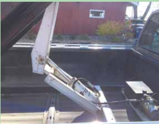
He cut off part of a small grain cart and attached it to a home-built hoist mounted in the pickup bed. A swing dump gate on back opens up when cart is hoisted.
