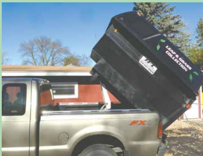
He cut off part of a small grain cart and attached it to a home-built hoist mounted in the pickup bed. A swing dump gate on back opens up when cart is hoisted.
