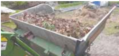
Peter Maitland uses a loader-mounted giant bucket to scoop up leaves in his yard. He built it by cutting up an old fiberglass boat.
