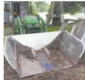
Peter Maitland uses a loader-mounted giant bucket to scoop up leaves in his yard. He built it by cutting up an old fiberglass boat.
