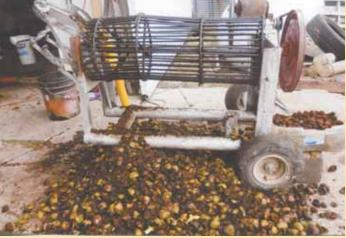
Rotating, cylinder-shaped cage separates hulls from nuts, eliminating the need to do the job by hand.
