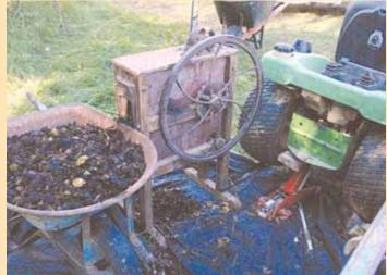
John Kocur used one of the wheels on a riding mower to friction-drive an old hand-cranked corn sheller. "It really works slick to crack walnuts," he says.
