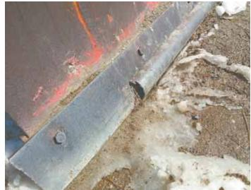
Greenberg mounted a length of steel pipe over the cutting edge of the blade on his skid loader. "The pipe lets the plow glide right over mud and rocks," he says.
