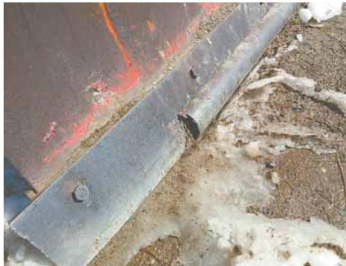
Greenberg mounted a length of steel pipe over the cutting edge of the blade on his skid loader. “The pipe lets the plow glide right over mud and rocks,” he says.
