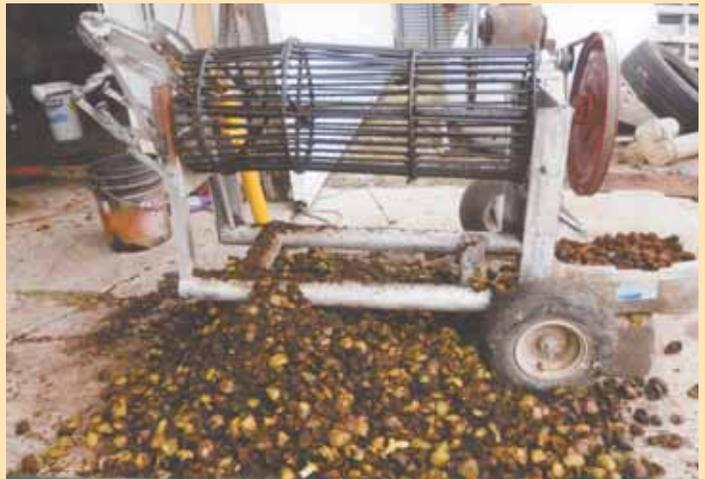
Rotating, cylinder-shaped cage separates hulls from nuts, eliminating the need to do the job by hand.
