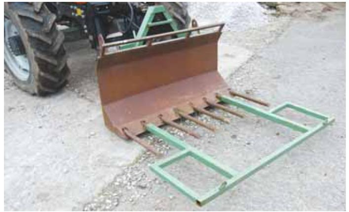
Alistair Robert used 2-in. box tubing to build this loader-mounted ATV hauler. The frame slips over 2 forks on loader bucket.
