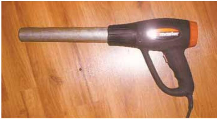
Dan Dodge used a 1,500-watt heat gun to make this “draft inducer” for his kitchen stove, adding a 10-in. length of thin-wall conduit to the end of the gun.
