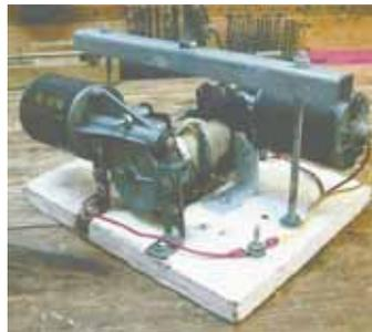
Salvaged power window motors drive mini-winch, which is equipped with a 3-in. long spool and high-strength webbing.
