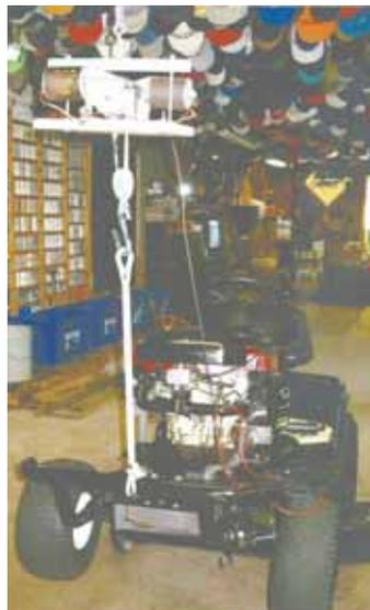
Krentz uses the mini-winch to lift spare tires into place, and to lift his riding mower for blade replacement.
