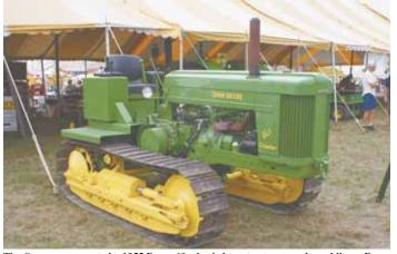
Tim Sweeney converted a 1955 Deere 60 wheeled tractor to a crawler, adding a Deere 2010 track and steering clutch assembly.
