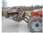
Two of the ATV's wheels fit into wells in frame.
