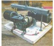
Salvaged power window motors drive mini-winch, which is equipped with a 3-in. long spool and high-strength webbing.
