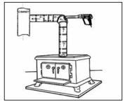
Heat gun slips into an oval hole cut into stove pipe elbow.
