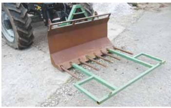
Alistair Robert used 2-in. box tubing to build this loader-mounted ATV hauler. The frame slips over 2 forks on loader bucket.
