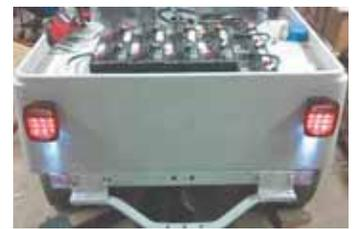
Lithium batteries would greatly increase the distance, but cost two to three times as much as standard batteries.
