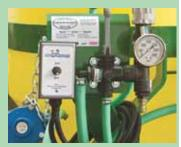
The operator uses a hand wand to spray fruit trees. Close-up photo shows sprayer controls, including pressure gauge and on-off pump switch.
