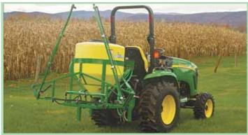
Alvin Wittmer's 3-pt. mounted sprayer comes with a 12 or 18-ft. boom that can be extended in 18 or 36-in. increments, and filled with an 80 or 35-gal. tank.
