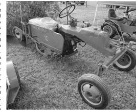
long wheelbase made it tippy when turning, so the company tried to compensate by installing front wheel weights. The tractor didn't come with a differential. Instead, it has a forward and reverse variable speed transmission that works like a snowmobile clutch. Levers at the base of the steering column are used to control the clutch and throttle. Other levers are used to lift the plow and to adjust plow depth."
