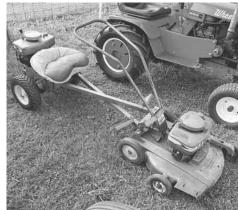
rode on pneumatic wheels. By replacing the deck with a pair of wheels, the operator could quickly convert the machine into a 4-wheeled tractor."
