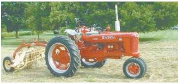
Indiana mechanic Bret Messer says putting a 4-cyl. Ford diesel engine into his Farmall H wasn't too difficult, once he figured out how to adapt the engine to the drivetrain.
