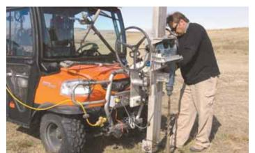
Gary Kehler uses seismoelectric technology to find water. He's shown here drilling a test shot hole with equipment mounted on his ATV.
