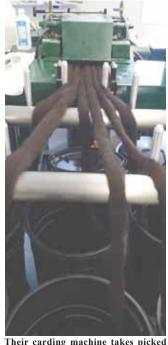
fibers and aligns them while removing dirt and foreign material.
