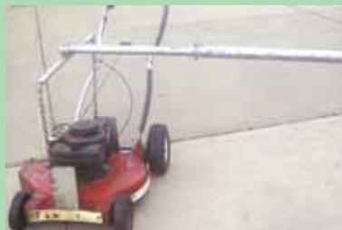
Side-mount hitch carries a 22-in. wide push mower about 10 ft. beyond the bucket on James Rohr's loader tractor. Chains attached to mower deck allow it to roll easily over uneven ground.
