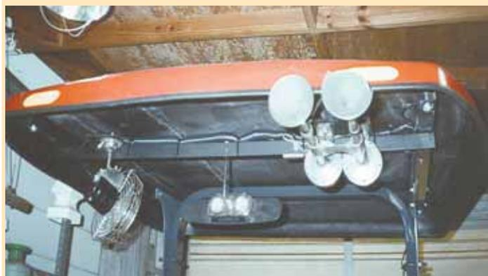
A 12-volt fan keeps Howard Aul cool inside his Kubota 4-WD diesel tractor. Fan mounts on a length of tubing that also supports a pair of electric horns.
