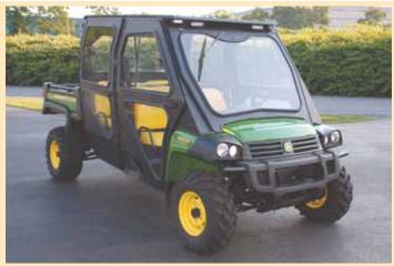
Curtis Industries recently introduced this commercial steel and acrylic cab for Deere's 4-door, 4-passenger Gator. Cab's lockable doors can be removed in seconds.
