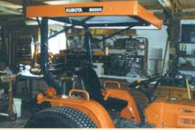
Homemade canopy is made from plywood, with pine 1 by 4's around the sides. It bolts onto Kubota tractor's rollbar.
