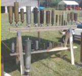
shells ranging from 75 to 105 mm. A pipe with elbows and an air compressor hookup connects the shells together. They are designed to make a triple tone like you find on big ships.
