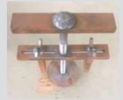
Steve Bellaw built this clutch spring compressor for an automatic transmission that needed to be rebuilt.
