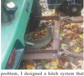
problem, 1 designed a hitch system that supports the motor and fastens to the vac with two 1/2-in. bolts and a 3/4-in. dia. hitch pin. The hitch pivots up and down and twists back and forth. All the metal came from an old hay rake, including the curved brace that connects with the hitch pin."
