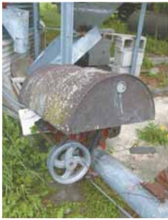
**David Obrecht, Zearing, Iowa:** To protect the electric motor on his bin auger from the weather, David cut a 55-gal. drum in half and mounted it over the top of the motor.
