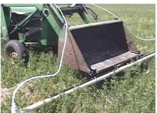
Weed wiper comes in sections 6 to 10 ft. wide that clamp onto loader bucket.
