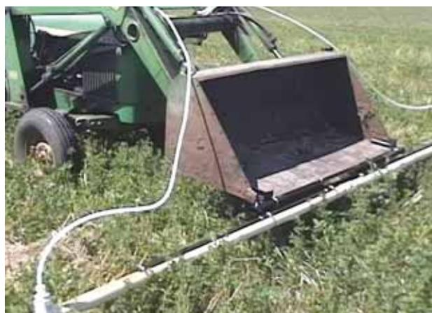
Weed wiper comes in sections 6 to 10 ft. wide that clamp onto loader bucket.
