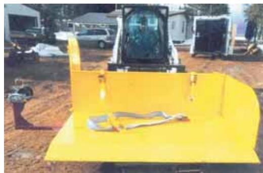
Carrier's end pieces are hinged at the bottom and can be swung back out of the way, allowing you to load the cow from either side.
