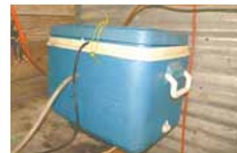
Water is pumped from a cooler filled with water and 2-liter bottles of ice.
