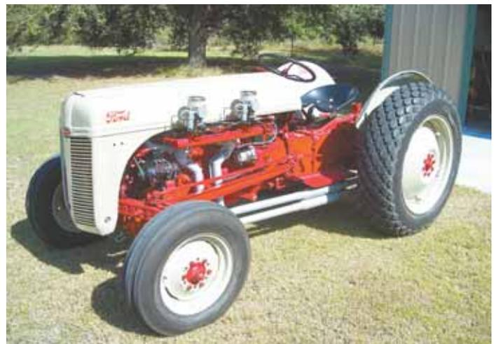
Charles Scudder repowered his Ford 8N with a straight-8 engine out of a 1951 Buick. "I had to have the engine rebuilt by a machine shop, but I did everything else," he says.
