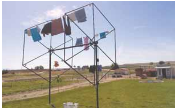
Clothes attach to wires strung between a pair of hexagon-shaped wheels attached to an axle. Operator turns a crank to rotate the wheels.
