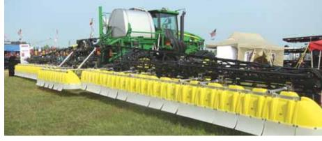
Hooded retrofit kit is designed to fit specific self-propelled sprayer models including certain Deere, Case, and RoGator models.
