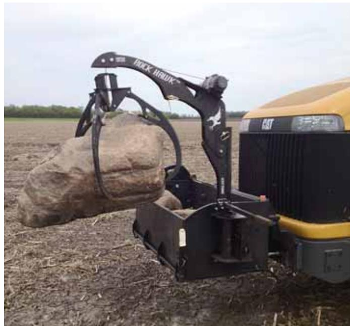
Rock Hawk bolts onto any rock box and works like a small crane. It lets you pick up big rocks in the field and then swing them over into the box.
