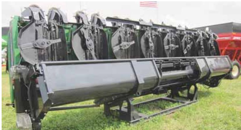
Geringhoff's stover collecting header allows you to harvest corn while creating a clean windrow of stover at the same time. Chopper blades cut the stalks into small pieces and send them flying into an auger, which drops them from a 5-ft. wide opening at middle of header.
