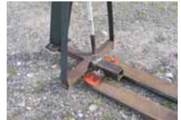
Photo shows how engine hoist mounting plate and hitch socket fit onto tractor forks.
