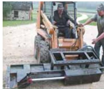
There are 3 splitting options. Above photo shows the I-beam laid flat to split wood on the ground.
