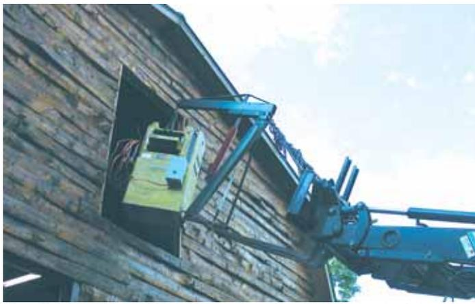
Glenn Haley recently used his loader tractor and modified shop engine hoist to lift a 500-lb. wood planer up into his barn's loft.
