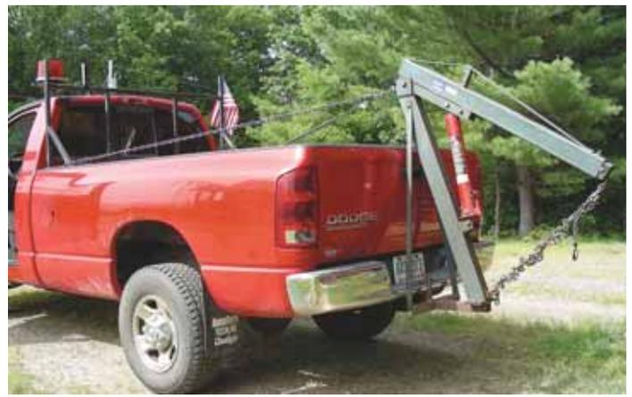
He can also use the hoist on back of his pickup. Chains are used to brace the hoist on both the pickup and tractor.
