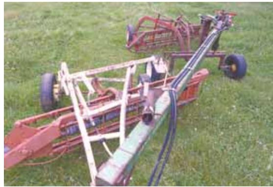
Christians used scrap steel to build 2 hitches and welded one to the main bar and the other one to the wing.
