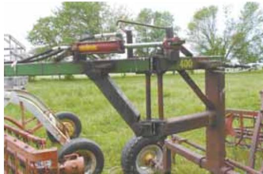
A double acting hydraulic cylinder at the pivot point is used to move the back rake from one side to the other.
