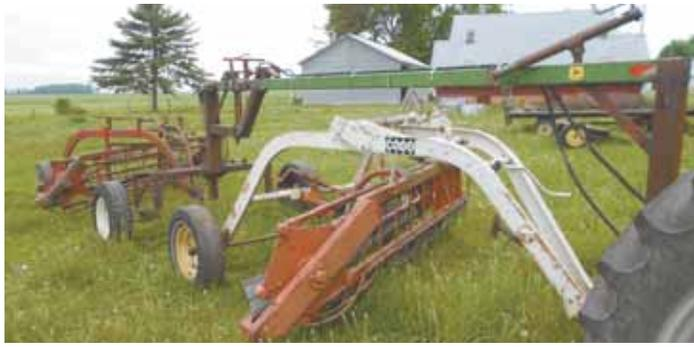
Minnesota farmer Jason Christians built this twin rake hitch from the frame of a mounted rotary hoe and wheels off a self-propelled combine.
