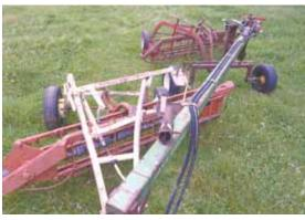
Christians used scrap steel to build 2 hitches and welded one to the main bar and the other one to the wing.
