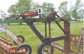
A double acting hydraulic cylinder at the pivot point is used to move the back rake from one side to the other.
