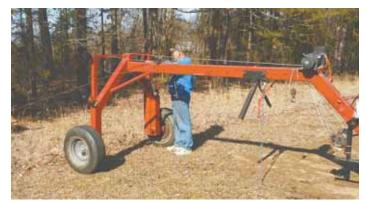
Winch mounted on top of arch pulls logs out of the woods.
