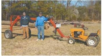
Euart log arch is fitted with a standard ball receiver hitch.
