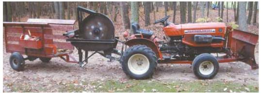
Almost everything Jerry Johnston brings to the woods to cut firewood is home-built and designed to work with his Yanmar 4-WD, 16 hp tractor. Equipment includes a 3-pt., pto-driven buzz saw, a log splitter, and a wood-hauling trailer that pulls behind either machine.
