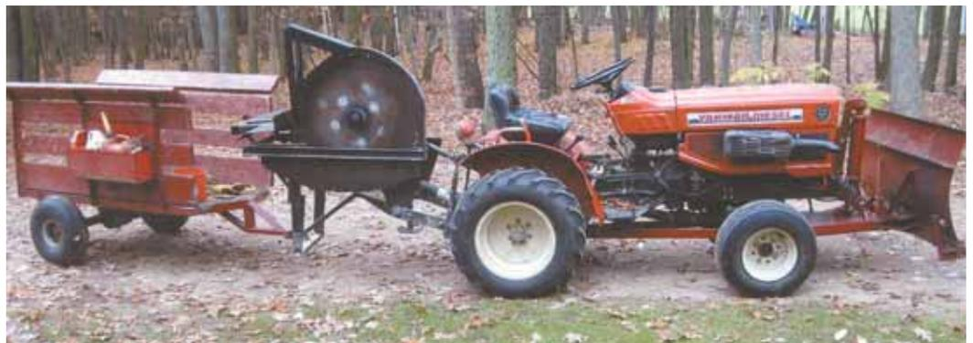
Almost everything Jerry Johnston brings to the woods to cut firewood is home-built and designed to work with his Yanmar 4-WD, 16 hp tractor. Equipment includes a 3-pt., pto-driven buzz saw, a log splitter, and a wood-hauling trailer that pulls behind either machine.
