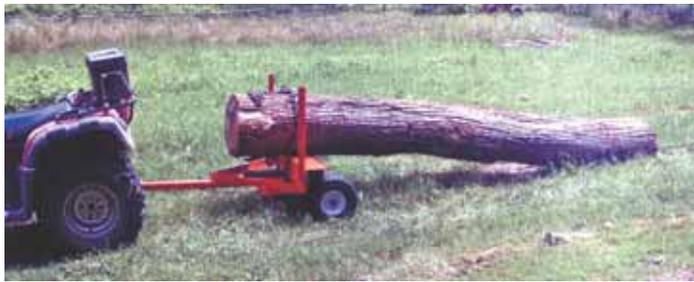
Log skidder rides on 13-in. flat-free tires that support a steel shelf 2 ft. above the ground. A 2-ft. steel upright bolts onto each side of shelf.
