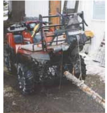
Allison uses a remote control to operate the winch. “It can handle logs up to 600 lbs.,” he says.
