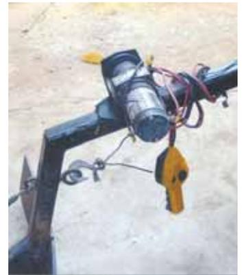
Logging arch slips into a 2-in. receiver hitch on back of Allison’s 4-wheeler and is fitted with an electric winch.
