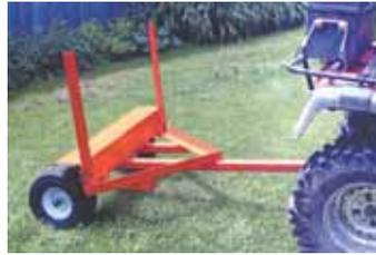
Each upright is secured by a double-nutted bolt with a pin 2 in. above it. By removing the pin, Irwin can lower the upright to the ground to form a ramp on either side.
