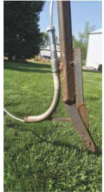
A curved 1-in. dia. tube clamps on behind 3-pt. trencher to feed cable down into trench.
