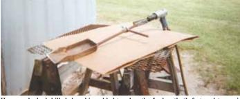
Homemade duck-billed shovel is welded to a length of rebar that's fastened to an air hammer. Hackman recently used the shovel to dig an 8-in. deep trench in hard ground.
