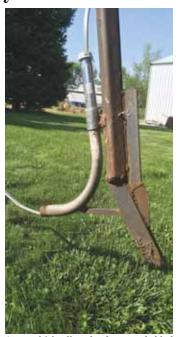
A curved 1-in. dia. tube clamps on behind 3-pt. trencher to feed cable down into trench.
