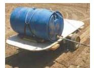
A 3-ft. long "boom" extends out one side of the 2-wheeled trailer.
