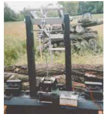
Grapple fork is opened and closed by a rocker arm mounted between two uprights.
