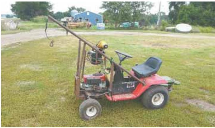
Cody Powell converted his MTD riding mower into a garden tractor "tow truck". An electric winch mounts in front of the steering wheel within reach of the driver.
